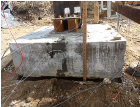
Figure 89. Soil rounding. (a) Parameters of CIM; (b), (c) Measurement of uplift amplitude and contact length during testing.
